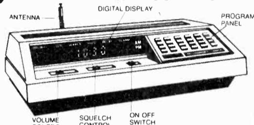
The Regency Z30 is a compact, programmable 30 channel, multi band, FM monitor receiver for use at home or on the road. It is double conversion, super heterodyne used to receive the narrow band FM communications in the amateur, public safety and business bands: 30-50, 144-174, and 440-512 MHz. Size 10 3/4" W x 2 7/8" H x 8 3/8" D.
