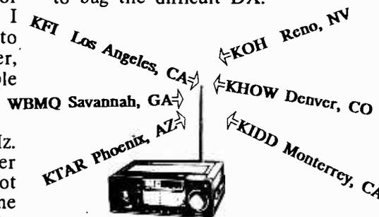
Let's say for some reason you've targeted WBMQ-630 Savannah, GA as your next DX target. You've taken care of projected interference from KOH-Reno, NV; KIDD-Monterrey, CA; and KHOW-Denver, CO by using a beverage antenna pointed directly east at Savannah from Los Angeles, your QTH, knowing that most signals from other directions will be attenuated. What other plans will you need to make?
