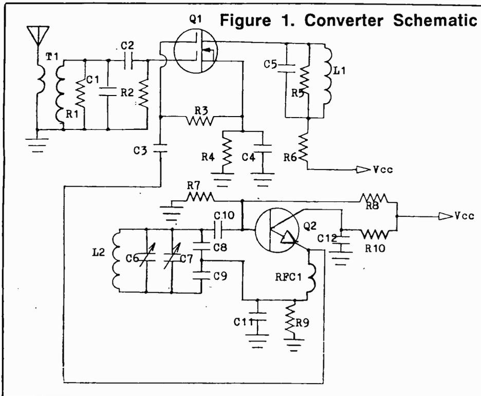
6.8 to 7.25 MHz. After you've done this, and before going any further, glue the coils of L2 into place.
