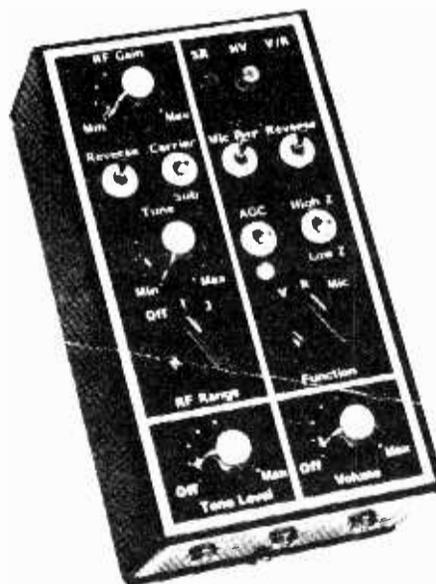
Bug detectors come in many forms: The ACM-2 Countermeasures Instrument pictured above aids in the detection of hidden microphones, carrier current transmitters, hidden tape recorders, concealed video cameras, telephone taps and bugs, telephone eavesdropping modifications, visible and infrared light attacks, and RF subcarriers. Easier for the novice to operate is the "Superhound" by Ross Engineering, pictured on the right.
