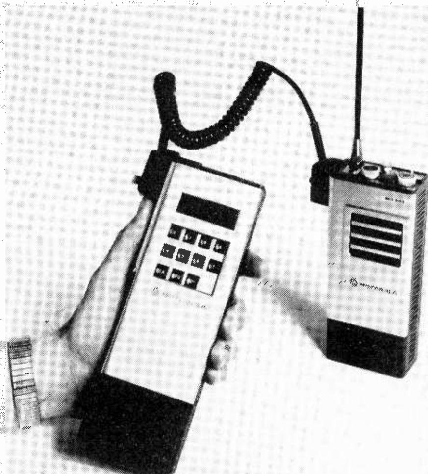
A special DVP code-inserter programs a specially-equipped (MX-series) hand-held for voice security (Courtesy of Motorola)
