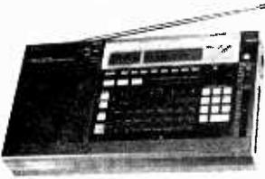
*"Sony's ICF-2010 represents a qualitative advance over conventional radios. It's the first widely-distributed receiver to operate in the synchronous exalted-carrier selectable sideband (ECSS-s) mode... to reduce interference and distortion far more effectively than can a conventional shortwave radio"*
