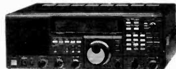
150 kHz - 29.999 MHz. 12 Memories. Optional 118 - 174 MHz converter. AM, FM, SSB, CW. LCD readout. Scanning. 2 Clocks/Timer.
