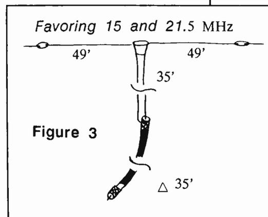
Tape twinlead, coax junction well for strength and water proofing.
