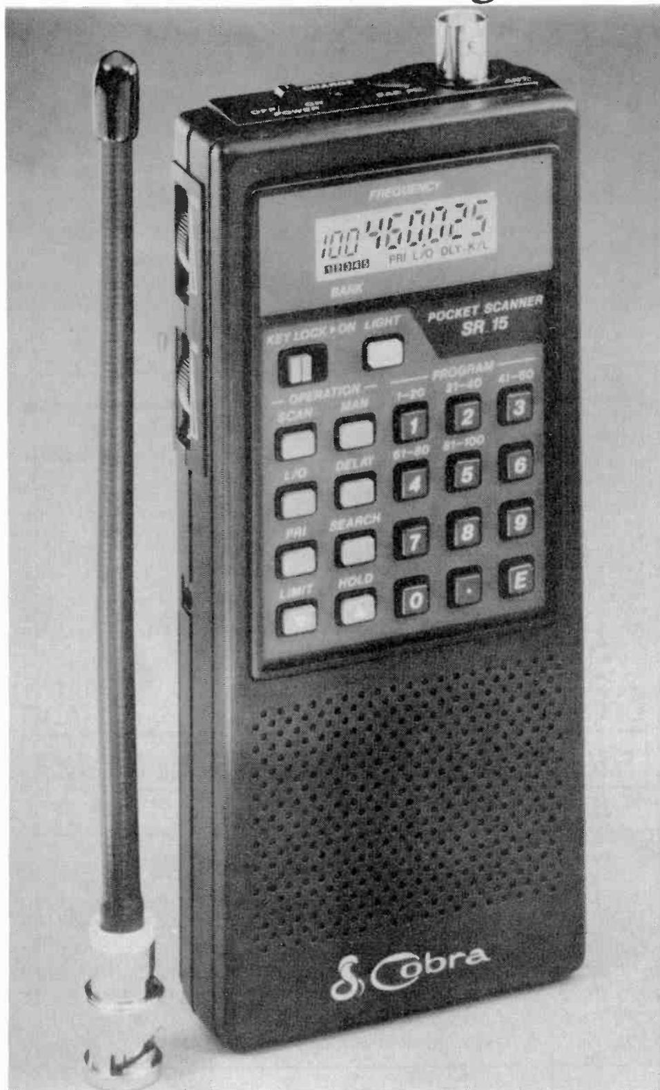
One of the newer additions to the ever-growing number of "mega-channel" handheld scanners is the Cobra model SR15. Measuring a scant 2-3/4"W x 6"H, and weighing only 10- 1/4 ounces, this one truly meets the meaning of a "pocket scanner." Its small size, coupled with its 100 channel capability, make the SR 15 quite versatile.
