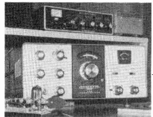
Photo 2: W3AZR spent \$75 on this Elmac AF-67 transmitter and Heath HR-10B receiver. 160 to 10 meters CW/AM and NBFM; and take a look at those dandy DX QSL cards on the wall!
