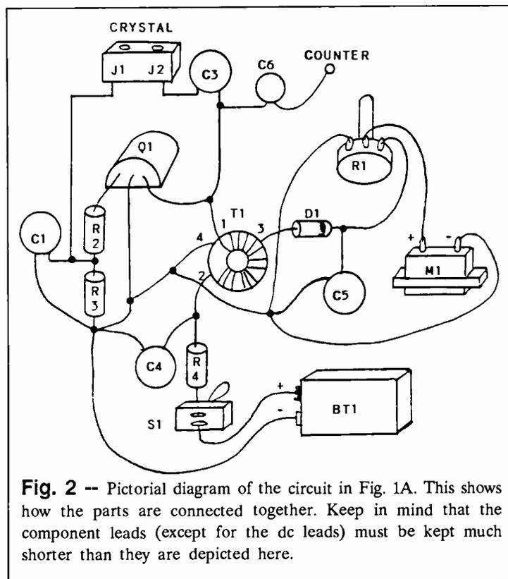
Fig. 2 -- Pictorial diagram of the circuit in Fig. 1A. This shows how the parts are connected together. Keep in mind that the component leads (except for the dc leads) must be kept much shorter than they are depicted here.
