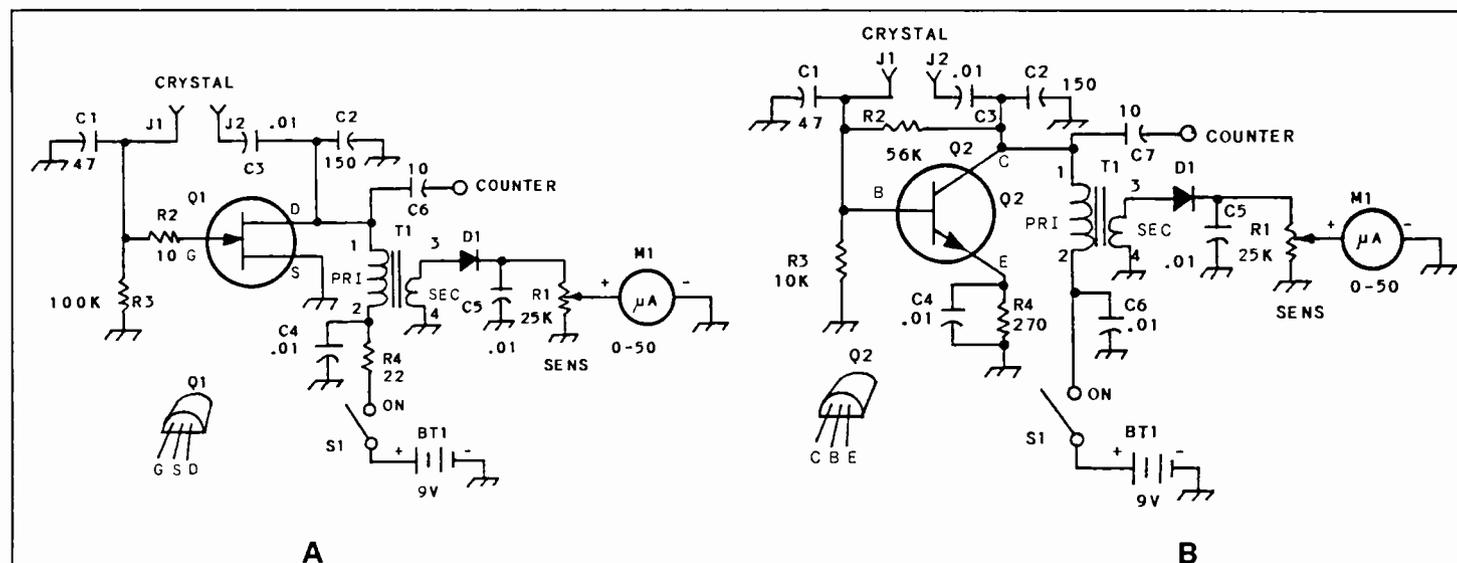
Fig 1 - Schematic diagrams of two crystal testers.
