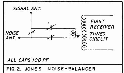
If you don't want to dig into the innards of your rig, this circuit should also work with its center-tapped coil positioned around the tuning coil in your antenna tuner, if you happen to use one. Experimenting with the number of turns and coil placement is likely to improve performance of the circuit. One note of encouragement: patience and perseverance are said to be essential when working with noise-balancing circuits.
