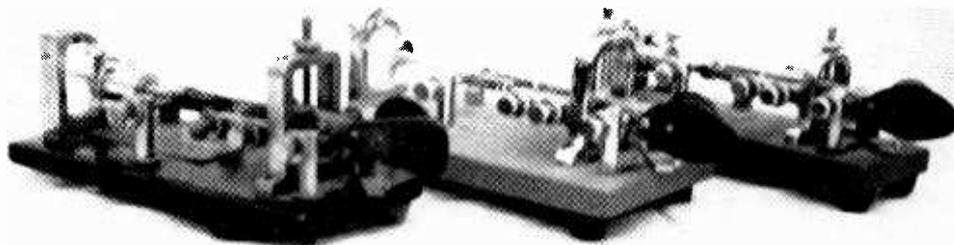
Three of the famous Vibroplex bugs; On the left is an early model (appears to have been a prototype). It is about 60 or more years old. Next is an Original which is the most popular of the Vibroplex line. And on the right is a compact bug called a Blue Racer.
