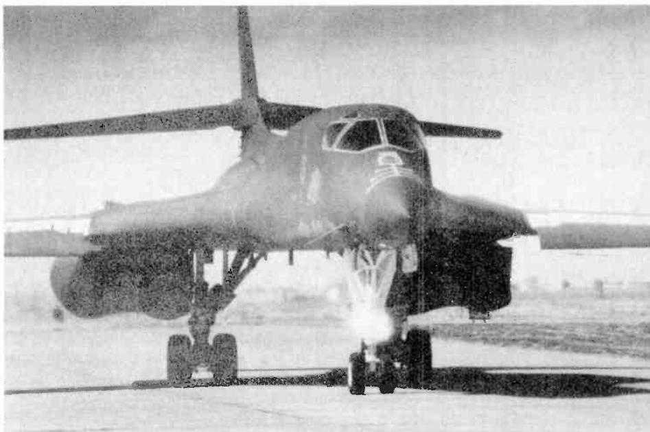
B-1b bomber from Ellsworth AFB South Dakota. The B-1b was designed with Stealth characteristics in mind but depends on a sophisticated electronic spoofing package to survive.
