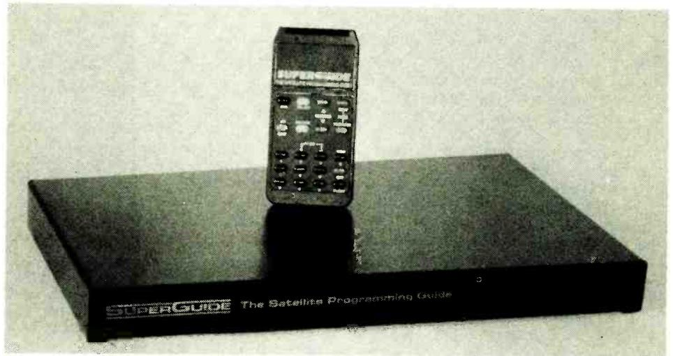
Stand-alone receiver with IR-RC for SuperGuide by Triple D Publishing. The electronic satellite guide is delivered to the customers' homes via satellite and displayed on any TV set or video monitor.
