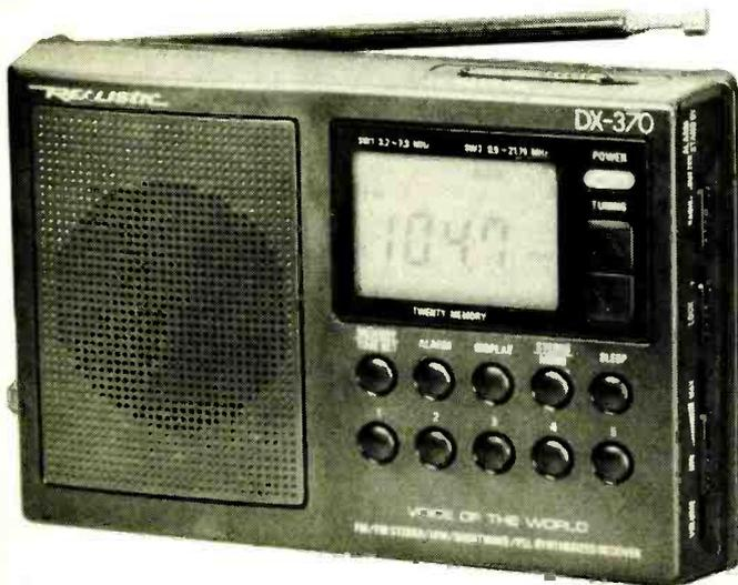
That digital display, although it's not illuminated, has good contrast and fairly large numbers. However, it uses the XX.XXx MHz format, rather than XXXXX kHz. To boot, the least-significant digit doesn't appear if it's a zero. So, for example, 15360 shows as 15.36. Again, a petty annoyance that you grow accustomed to.
