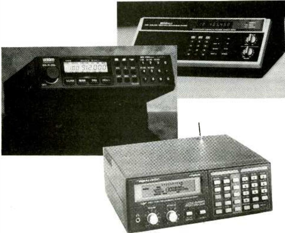
could well be the best scanner ever made. Its 400 memory channels are enough for just about anyone; user-selectable AM, FM wide and FM narrow modes provide additional -- and useful -- functionality. Frequency coverage of 25-520 and 760-1300 MHz (cellular excluded; easily restored) meets most anyone's needs.
