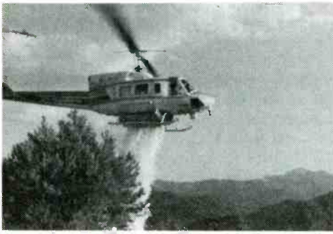
Helicopter pilots making belly drops of water on fire spot have a hard time seeing the target and are guided via air/ground radio.
