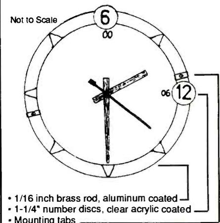
The outer ring is 13-1/4" in diameter; the inside ring is 12-3/4". Number disks are cut from white poster board and numbers are black applied with a lettering guide. After mounting on the frame with epoxy cement, they are sprayed with clear polyurethane. The finished assembly mounts on the raised rim around the face of the clock with two small self-tapping screws. There are two sets of mounting holes allowing the number ring to rotate when changing from Daylight to Standard Time.
