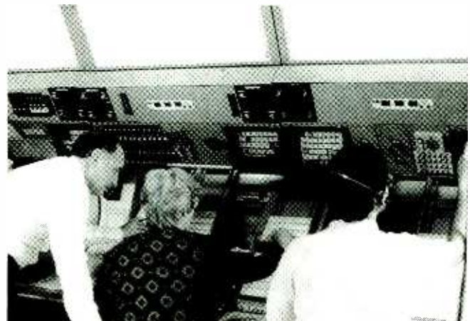
The VSCS system in operation at a simulated Air Route Traffic Control Center. Screens are dark until the controller plugs in a headset.
