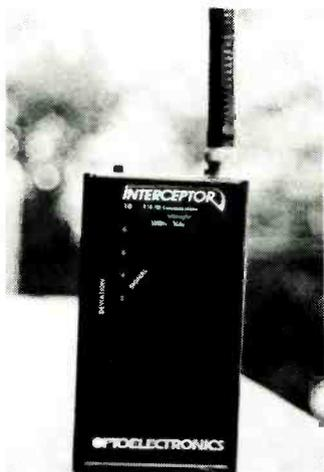
The "Interceptor" is a high tech instrument that can monitor between 30 and 1000 MHz.
