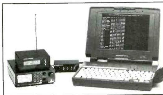
**Ideal For Testing Two Way Radios** can be directly connected to the Model R10 Interceptor™ for checking CTCSS, DTMS, Deviation, Signal Strength and Audio. **Update older service monitors.** **Unique features** such as an actively decoding indicator squelch connection, a serial communications
