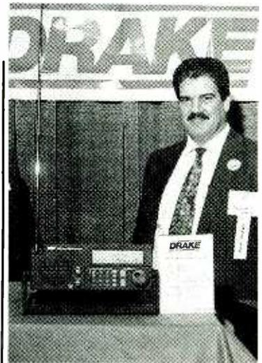
Coverage is 5 kHz to 30 MHz, with superior IF digital filtering, multimode reception, RS-232 or CSMA remote control, and more.
