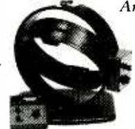
Air-core design - tunes 530 to 1700 kHz with variable bandwidth (2 kHz to 15 kHz), gear reduction for precise nulling of signals, liquid filled compass for bearing measurements and more!
