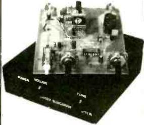
Tap into the world of commercial-free music and data that is carried over many standard FM broadcast radio stations. Decoder hooks to the demodulator of FM radio and tunes the 50-100kHz SCA subcarrier band. Many radios have a demod output, but if your radio doesn't, it's easy to locate, or use our FR-1 FM receiver kit which is a
