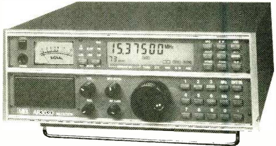
non-standard configuration: a 3 x 3 setup, with the "1" at upper left, and the zero offset to the right of the "9." Fortunately, the software is relatively friendly. To enter 5975 kHz, just press 5, 9, 7, 5, and kHz, and it's done.
