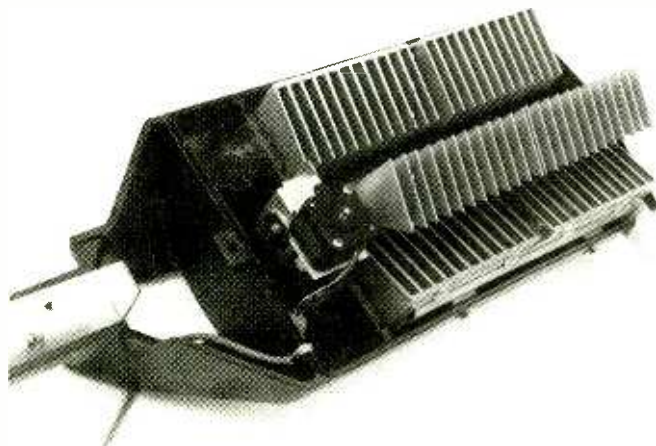
AEA IsoLoop antenna with case off and large capacitor
