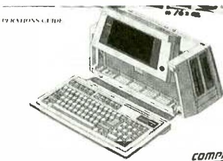
How can we use the ten year old, 286, 12 MHz, plasma screen computer shown in Figure 1? Let's see. Although the Compaqs have 40 Megabyte hard drives, they only came with 640k of RAM. Remember the days when that was the standard? Circa 1987. That was before Bill Gates impressed Windows 3.1 on the world. The non-standard memory type and arrangement used by Compaq makes memory expansion relatively expensive. Therefore, as they stand, we can only use the Compaqs to run DOS applications.
