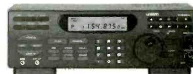
This popular, low cost scanner features wide frequency coverage (29-54, 108-174, 216-512, 806-956 MHz—less cellular), 200 memory channels, 100-channel-per-second TurboScan, weather alert, CTCSS (optional), channel activity counter, 10 channel priority, search autostore, tape recorder output, memory channel transfer, and much, much more!
