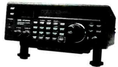
reception (AM/FM/LSB/USB/CW), selectable IF bandwidths (3/6/15/40/110/220 kHz), superb frequency stability (+/-1 ppm, 0-50 deg. C.), mobile or fixed power (12 VDC / 120 VAC), and much, much more. See detailed specifications on pp. 8-9.
