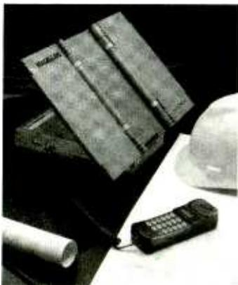
Bob Grove set up the Magellan MicroCom-M satellite telephone on an old picnic bench in the middle of the North Carolina woods. The thing is remarkably easy to get going. You turn the unit on, unfold the two panels that act as the antenna, and point it at the nearest satellite. (You know when you're on target by watching the LED light bar.) All that's left to do is to pick up the handset and dial!
