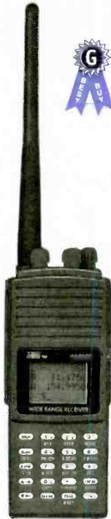
With wide frequency coverage—500 kHz-1900 MHz (less cellular), 1000 memory channels, AM/FM/SSB reception, selectable tuning steps from 50 Hz-999.995 kHz. An oversized, edgelit LCD window holds 44 bold alphanumeric characters.
