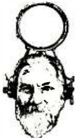
I assume that that's Mr. Judd in Figure 1, wearing his invention! Figure 2 shows the construction in more detail. The eight-inch tuning coil is wound "duo-lateral-wise," a 20 plate, 250 micro-microfarad tuning capacitor is mounted in one head phone—with a knob, and a crystal detector is mounted on the outside of the remaining headphone, which contains a 2,000 ohm receiver Figure 3 shows the simple wiring for this very unique receiver
