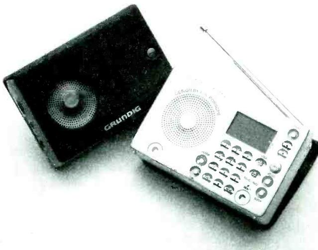
*When you want to use the radio, you simply flip over the front part of the case so it clings magnetically to the back. Not only does this get the case out of the way, it also allows the case to serve as an elevation panel to place the radio at a handy angle for operation.*
