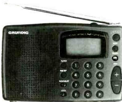
With the Grundig Traveller III, there is no dialing—ever. To search any broadcast band use Auto Scan and the Traveller III stops at the next station. Twenty memories store your favorite stations for instant retrieval at the push of a button. Plus the digital-display clock is quartz-accurate.
