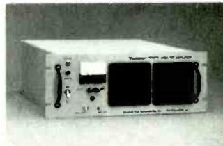
The 500A employs a closed-loop negative feedback circuit which ensures a low-output impedance (close to zero ohms). Full power is obtained with a load resistance of 1.25 ohms and 25 volts rms output voltage. However, any other combination of voltages (up to 15,000) and current (up to 200 amps) can be obtained through the use of an optional transformer. The 500A is fully protected against overloads and overheating.
