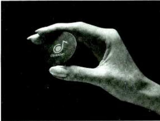
*Don't throw that little plastic chip away! That's your satellite antenna, downconverter, and 900 MHz wireless relay to your in-dash satellite receiver. (Courtesy CD Radio, Inc.)*
