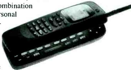
The 13.9 ounce Communicator is first a fully-featured 1900 MHz GSM telephone with all the features PCS subscribers have come to expect, including Caller-ID and short messaging. Opening the unit lengthwise reveals a compact QWERTY keyboard and a liquid crystal graphics display. A call in progress will automatically be switched to the integrated speakerphone, freeing the user to take notes or perform other computer operations.
