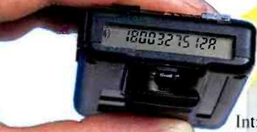
Introducing the all new Techtoyz Micro DTMF Decoder. The Micro DTMF Decoder, housed in a pager style case, is ideal for portable, hands free operation. With its built-in microphone, DTMF tones are automatically decoded from the signal source of tape recorders, receivers, two-way radios, etc... Tones are displayed on the Micro Decoder's 12 digit LCD display and automatically stored in the 2000 character non-volatile memory for review.
