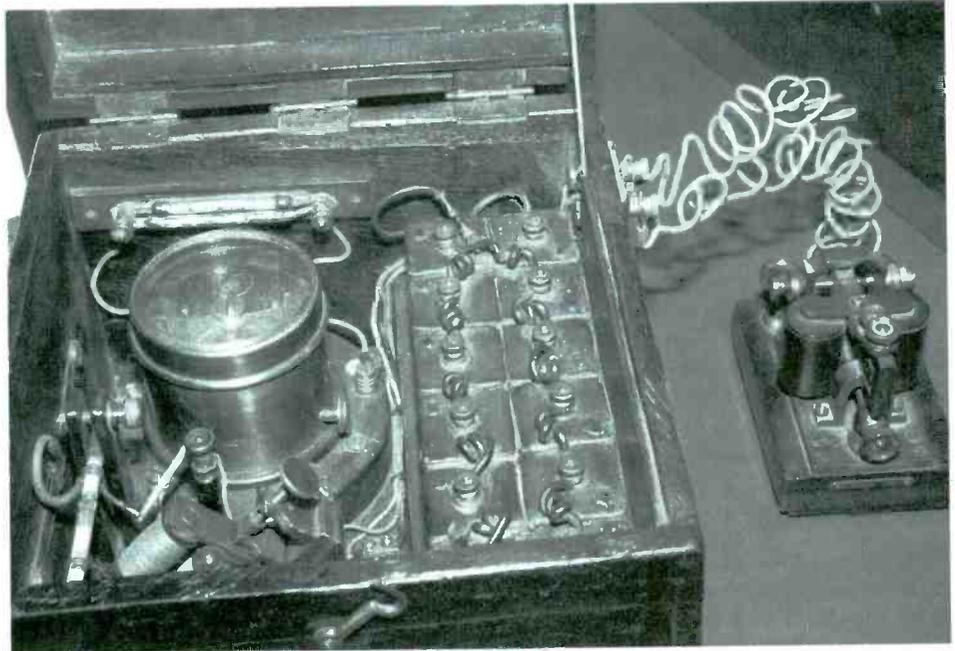
*The inside of a Marconi receiver of the type used in his London GPO demonstration, 1896.*
