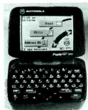
The user can receive messages, respond to those messages, and initiate customized messages. An Intel microprocessor and a software development kit (SDK) allow programmers to use industry-standard development tools to create additional applications.
