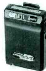
Four modes of operation—Normal, Filter, Recall, and Digital Auto Capture—allow the user flexibility in using the counter. Only three internal memories are provided for logging captured frequencies, however.
