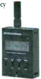
Connected to any scanner with a CI-V interface, allows automatic reception of any intercepted signal within the scanner's frequency range. For use with the AR8000, order SAC-8000; for the R10 order ADPK-4; for R7000, R7100, R8500, R9000, use ACC-74 or ACC-157.
