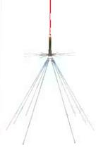
The discone antenna is used by government and military agencies worldwide because of its wide bandwidth characteristics and non-directional coverage. The Diamond D130J discone consists of 16 rugged, stainless steel elements and is capable of transmitting up to 200 watts above 50 MHz, and provides continuous 25-1000 MHz (and above) reception. Accomodate any standard mast-pipe (1" to 2-1/8" diameter).
