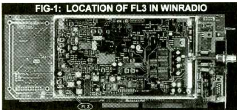
See "Step by Step" instructions for replacement of FL3, shown at lower left.
