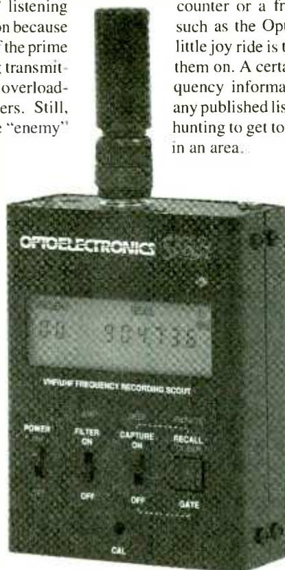
The Optoelectronics Scout is an ideal tool to "cruise" for new frequencies
