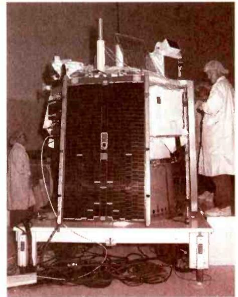
*Above: Johns Hopkins University engineers install solar array panels on the ACE spacecraft.*
