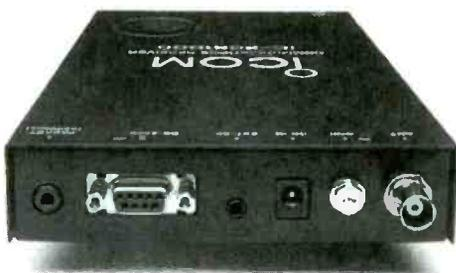
FIGURE 1 - IC-PCR1000 Back Panel
