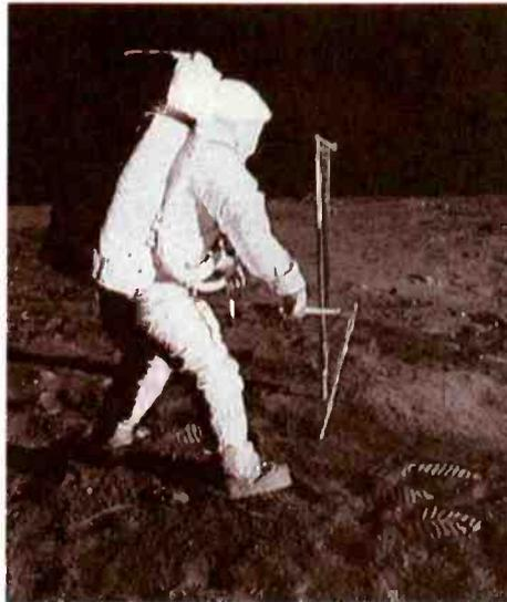
*An early attempt to analyze the solar wind was performed on the Apollo moon missions. Sheets of extremely pure aluminum were hung like window shades to collect particles from the solar wind. The sheets were carried back to the earth, cut into small samples, and analyzed by mass spectrometers.*
