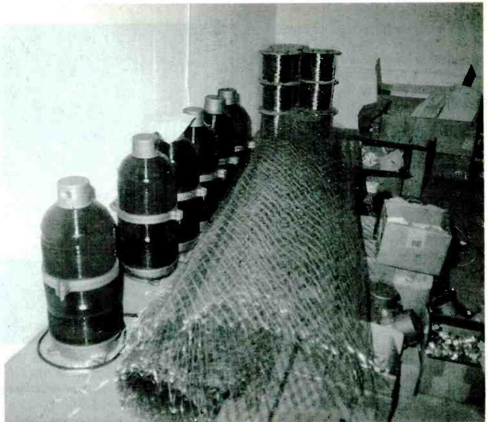
*Materials for an AM tower include a set of lights and a roll of wire mesh which is part of the grounding system.*
