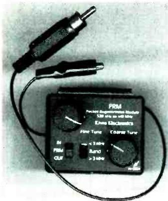
such as in this month's article on "Car DXing." However, you can boost the pocket-loop's reception by 18 dB of frequency-selective gain with the addition of the Pocket Regeneration Module. It works on frequency ranges from 530 kHz to 10 MHz.
