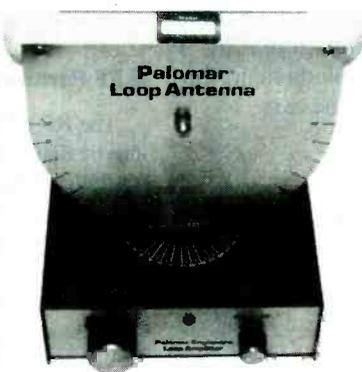
The Palomar Loop Antenna is an active antenna system which covers from 10 kHz to 16 MHz. Coverage of this very sizable chunk of RF spectrum is made possible by use of a different plug-in loop antenna element for each band. These loops are mounted such that they can be rotated to null-out undesired signals or noise.
