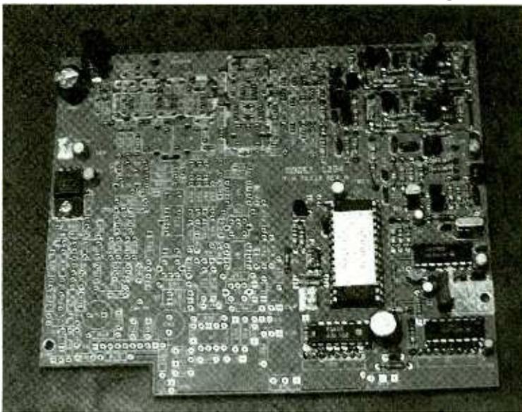
and cuts down on moving parts when you turn the board over to solder it. I also mounted all the resistors in all phases with the same orientation. This makes it easier to read the values and also will help you troubleshoot later if you put a resistor in the wrong place(!).
