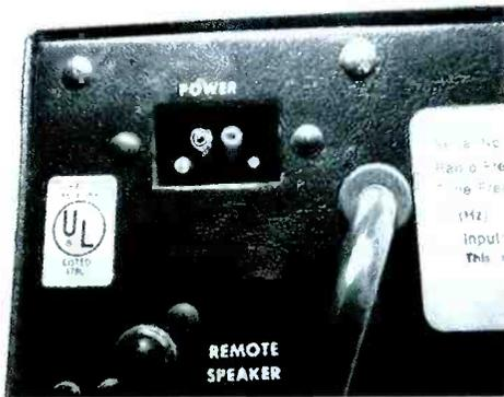
**FIGURE 3:** Permanent AC line cord installed through rubber grommet. Note insulation installed over top terminals on power connector to prevent shock.
