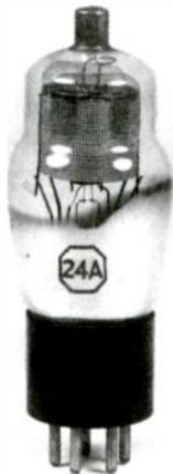
Fig. 1. Type 24-A was the first widely-used screen grid tube.
