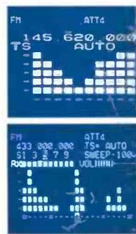
Signal strength (above) and band scope (below) functions assist in finding the action you want to hear...or see!
