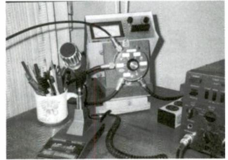
*Photo 7. By inadvertently selecting the wrong antenna, transmissions were sent out from the dipole at a three-foot high elevation.*
