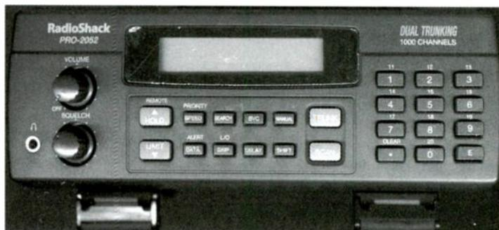
Figure 1: Radio Shack PRO-2052 scanner
