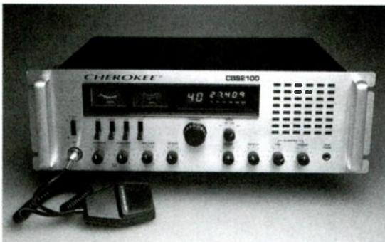
A compander circuit called Clear Drive compresses audio on transmit and expands it on receive. When both stations at either end of a conversation are using ClearDrive it can really boost the signal for long-haul communications, but the technology can also help in single station use as well.
