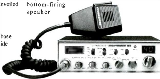
and connectors for antenna, public address speaker, external speaker, and power cord on the back panel. To boost performance under noisy conditions, it is equipped with Cherokee's Clear Drive system.
