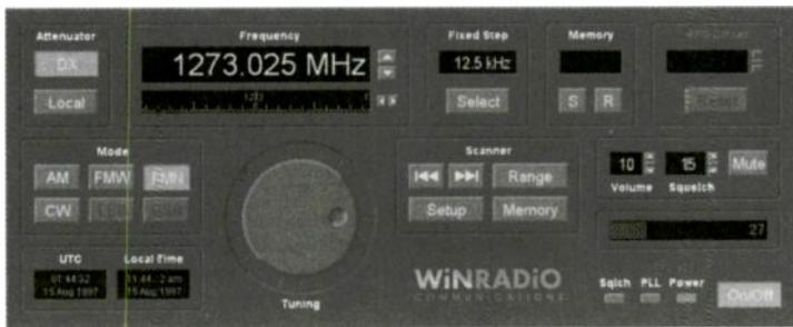
Looking for a computer-hosted, wideband receiver with better specs for signal surveillance? For starters, how about continuous 150 kHz-1500 MHz reception, 65 dB image and spurious signal rejection, and 85 dB dynamic range? This is the WiNRADiO WR-3150i-DSP, designed specifically for government, military, and law enforcement applications.
