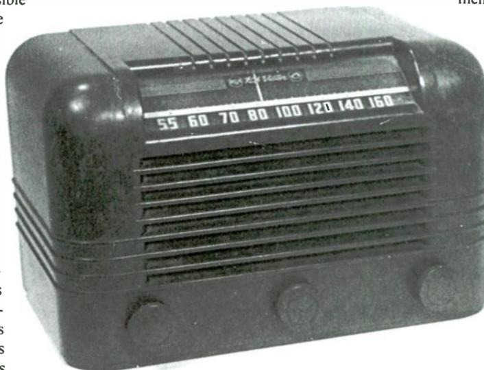
*The use of molded Bakelite made it possible to design cabinets with the sleek rounded lines favored by late 1930s industrial designers.*
