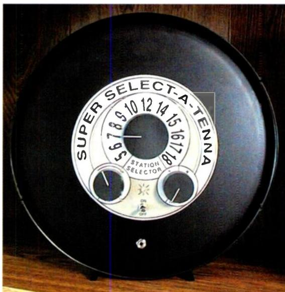
One of these applications involves coupling older model internal ferrite rod antennas that don't work well to this antenna to obtain good, high-Q, mutual coupling. My Sony 2010 tends to fit into this category and the Super-Select-A-Tenna did show a significant improvement over the second generation model I have been using with it.
