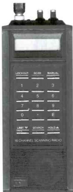
Figure 5. Electra Bearcat BC-100, the first programmable handheld scanner
