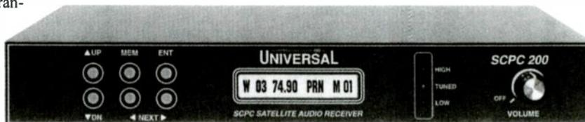
Universal's SCPC-200 receiver, a stand-alone SCPC receiver which features built-in companding, 50 channel memory, tuning LEDs, line or 8 ohm speaker output. (Courtesy Universal Electronics, Inc.)
