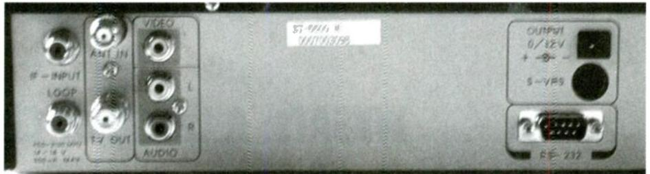
*There's not too much to do to get these receivers up and running. An LNB loop-through and video and audio output are all that are needed. There's even room for an outside TV antenna input.*
