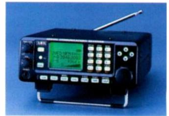
AR8600 can interface with your PC, display the spectrum, and scan or search at 37 channels per second. Five sockets receive optional function cards for extended performance. Operates directly from 12 VDC for mobile/portable applications, or from an AC adaptor. The AR8600 is expected to be available in November. Call Grove Enterprises for pricing and availability (800-438-8155) or visit Grove's new "Radio Rumors" page (see following).
