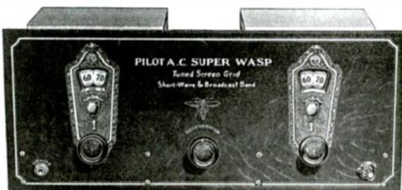
The A.C. Super Wasp's trim metal front panel has illuminated dials, simulated wood-grain finish. Cabinet was not included with set.
