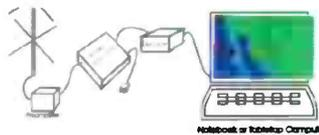
If you own an ICOM PCR1000, all you need for Weather pictures is an antenna, a preamplifier and a Timestep interface for your computer.
