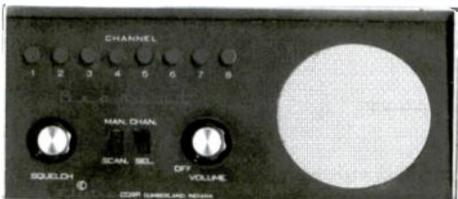
Figure 2. Electra Bearcat BC-L, first generation scanner.
