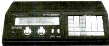
Figure 7. *Radio Shack PRO-2004 provided wide frequency coverage*
