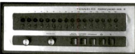
Figure 4. Tennelec Memoryscan MS2, code programmable scanner.
