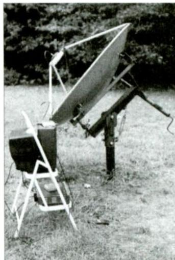
4.5' surplus spun aluminum dish with analog receiver using a C-band LNBF (courtesy author)
