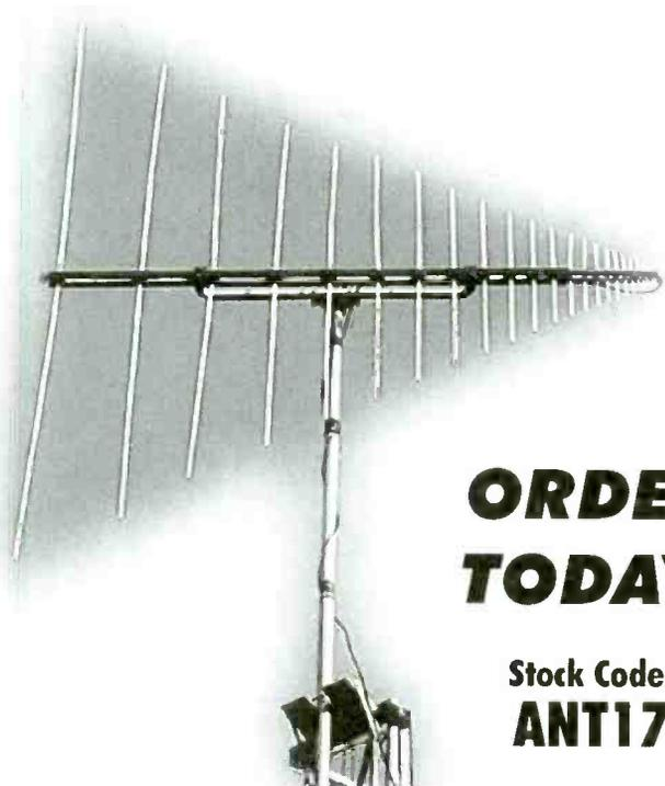
The log-periodic dipole array (LPDA) is respected for its wide bandwidth, constant impedance, and high gain. Measuring 4'10" boom length, the Create CLP-5130-2N (our catalog no. ANT-17) offers 100-1300 MHz bandwidth for transmitting and receiving, with an average forward gain of 11-13 dBi. Ruggedly constructed of solid aluminum for lightweight durability. Fitted with an N connector for low-loss coax.
