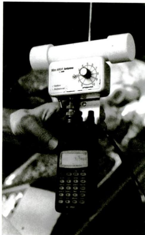
*For RDF on HF bands such as 80 meters, an external loop/sense antenna can be attached to a multi-mode hand-held receiver like the Icom IC-R10. Charles Scharlau NZØI of North Carolina made this one.*
