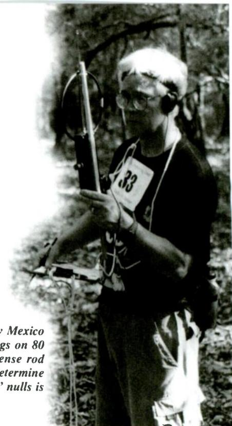
*Mike Pendley K5ATM of New Mexico uses an air loop to get bearings on 80 meters. Notice the vertical sense rod alongside the loop, to help determine which of the loop's "figure-8" nulls is toward the fox.*
