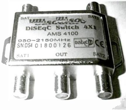
*DiSEqC switch allows switching between two fixed dishes and is done automatically through the ST-9900 receiver. (Courtesy: DVB Express)*
