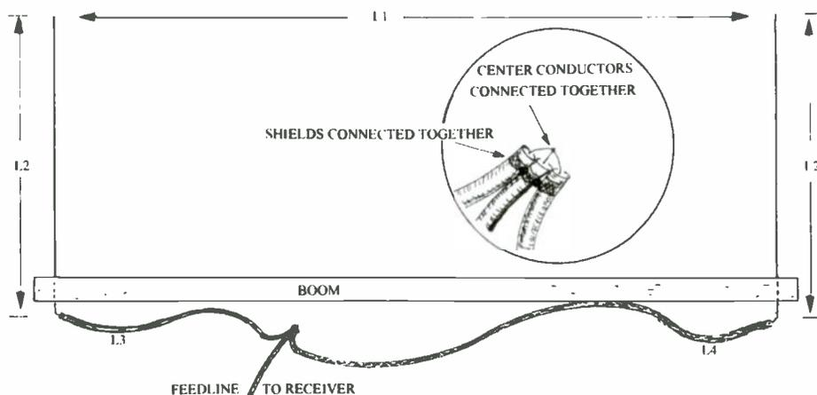
**Fig 1.** A phased array useful for RDF work. When connecting feed line and phasing lines, connect all shields together and all center conductors together as shown in the inset. At the vertical elements, only the center conductor of the phasing line is connected.
