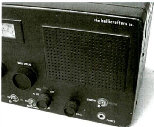
*Speaker grille of the S-40B is not a separate piece as in the earlier versions, but is formed from the metal of the panel itself. The "h" logo has been eliminated.*
