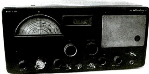
*S-40A front panel is in decent shape but needs freshening up. Trim ring is present on tuning knob (left, center), but missing on matching bandspread knob.*
