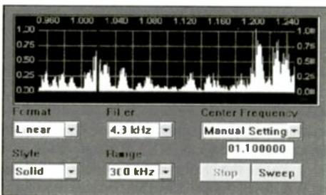
'Spectrum' (above) is a dandy little application that will quickly mute the radio, sweep it across a user-selected portion of the radio spectrum and plot the results in graph form. Here I chose the local AM band as an example. You can see just where the activity is and clicking on a peak with your mouse tunes the radio to that frequency.
