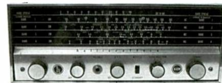
**Circuitry:** a.c.-d.c. superhet (no power transformer). No r.f. stage; one i.f. stage; bandspread; built-in speaker; BFO. Tube complement: 12BE6 oscillator/mixer; 12BA6 i.f. amplifier/BFO; 12AV6 detector, first audio amplifier, AVC; 50C5 audio output; selenium rectifier.
