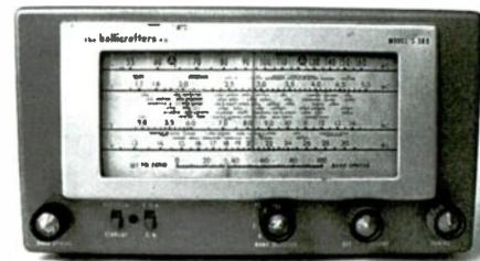
**Circuitry:** a.c.-d.c. superhet (no power transformer). No r.f. stage; one i.f. stage; bandspread; built-in speaker; BFO. Tube complement: 12SA7 oscillator/mixer; 12SG7 i.f. amplifier/BFO; 12SQ7 detector, first audio amplifier; 50L6 audio output; 35Z5 rectifier.
