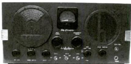
**Circuitry:** Transformer-powered superhet. One r.f. stage; two i.f. stages; bandspread; built-in speaker; BFO; noise-limiter; drift-compensated HF oscillator. Tube complement: 6SK7 r.f. amplifier; 6K8 oscillator/mixer; 6SK7 first i.f. amplifier; 6SK7 second i.f. amplifier; 6SQ7 second detector, AVC and first audio; 6H6 noise limiter; 6J5 BFO; 6F6 audio output; 80 rectifier.
