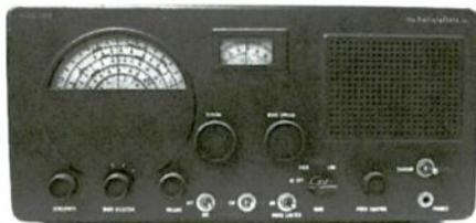
**Circuitry:** Transformer-powered superhet. One r.f. stage; two i.f. stages; bandspread; built-in speaker; BFO; noise-limiter. Tube complement: 6SG7 r.f. amplifier; 6SA7 oscillator/mixer; 6SK7 first i.f. amplifier; 6SK7 second i.f. amplifier; 6SL7 BFO/second detector; 6H6 noise limiter/AVC; 6F6 audio output; 5Y3 rectifier.
