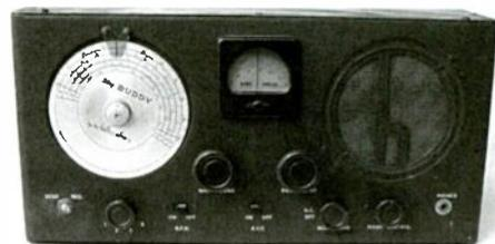
**Circuitry:** Transformer-powered superhet. No r.f. stage; one i.f. stage; bandspread; built-in speaker; BFO. *Tube complement:* 6K8 oscillator/mixer; 6SK7 or 6K7 i.f. amplifier; 6SQ7 or 6Q7 second detector, AVC and first audio; 41 audio output; 76 BFO; 80 rectifier.
