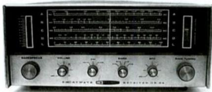
**Circuitry:** Transformer-powered superhet. No r.f. stage; one i.f. stage; bandspread; built-in speaker; BFO; noise limiter. Tube complement: 12BE6 oscillator/mixer; 12BA6 i.f.
