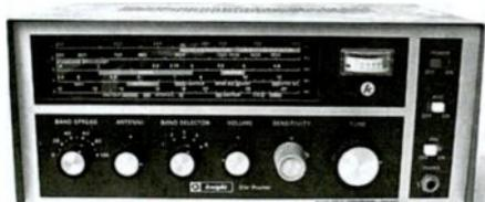
**Circuitry:** Transformer-powered superhet. No r.f. stage; one i.f. stage; bandspread; built-in speaker; BFO; noise limiter. Tube complement: 6BE6 oscillator/mixer; 6HR6 i.f. amplifier; 12AX7 detector, first audio amplifier; 6AK6 or 6AR5 audio output; semiconductor diodes.
