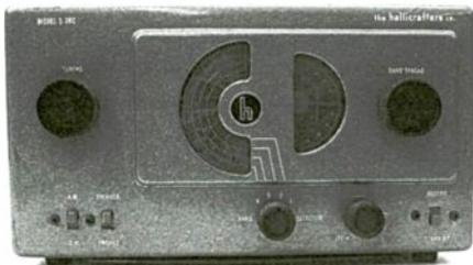
**Circuitry:** a.c.-d.c. superhet (no power transformer). No r.f. stage; one i.f. stage; bandspread; built-in speaker; BFO. Tube complement: 12SA7 oscillator/mixer; 12SK7 i.f. amplifier/BFO; 12SQ7 detector, AVC, first audio amplifier; 35L6 audio output; 35Z5 rectifier.
