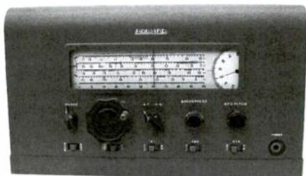
**Circuitry:** Transformer-powered superhet. No r.f. stage; one i.f. stage; bandspread; built-in speaker. BFO; noise limiter. Tube complement: 6K8 oscillator/mixer; 6SK7 i.f. amplifier; 6SQ7 detector, first audio; 6C5 BFO; 6H6 noise limiter; 6K6 audio output; 80 rectifier.
