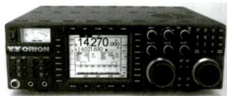
In addition to the incredible receiver dynamic range and brick wall filtering, the unit makes use of "Panoramic Stereo"™ that allows the user to pick out signals in a pile-up with ease.
