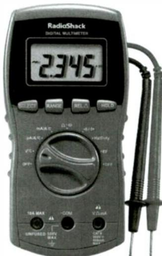
**Radio Shack's 42 Range Auto Ranging Multimeter (RS #122-811) sells for \$50. When you're ready to move to the intermediate level this multimeter also has auto-shut off and auto polarity. It measures frequencies to 4 MHz, detect electric fields, has a low battery indicator, and uses a common 9 volt battery. (Courtesy Radio Shack)**
