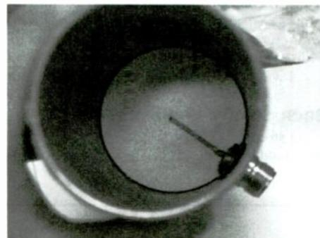
Figure 3: Connector installed on a Pringles can.
