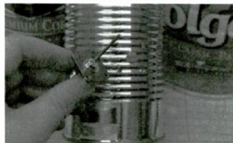
Figure 2: Connector with 1.21" wire attached.
