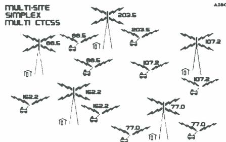
One drawback with multi-site simplex multi-CTCSS systems is that since *all* units share just one radio frequency, neighboring radio zone base stations and mobiles won't hear each other's traffic, but they will still interfere with each other. This means that as the amount of radio traffic in the *entire* system increases, interference increases and system throughput decreases.
