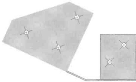
I put a 30° bend to conform to the installation location. Figure 5 shows the side view of what the finished product would look like.
