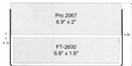
Second, I made drawings of the side-profile of each radio. After positioning the mounting points of each, I combined them into a profile of the two radios together, as they would be positioned when installed (fig. 2). I printed this out and cut off the excess paper to confirm that my initial configuration would actually fit where I thought it might. I got
