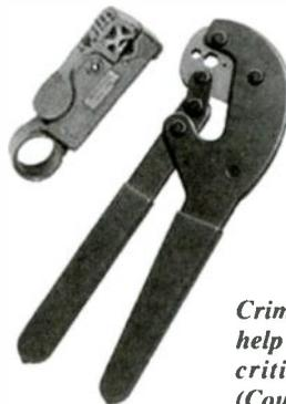
*Crimpers and strippers help do a perfect job on critical connections. (Courtesy Radio Shack)*
