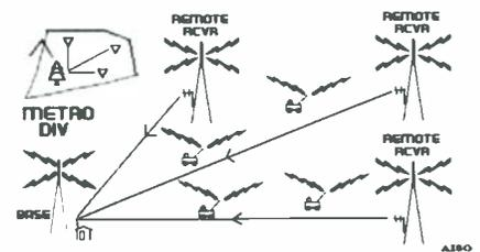
Some wide area radio systems can be quite complex, combining remote bases and remote receivers, and sometimes even having radio zones that have multiple sets of remote receivers linked to remote bases that are linked in turn to radio base stations.
