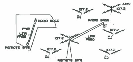
In areas where radio zone base stations cannot hear the mobiles but the mobiles can hear the base station, an unmanned remote receiver site is installed. It consists of a receiver only on the standard frequency for the radio zone and a remote link transmitter on another frequency that transmits back to the radio zone base station.
