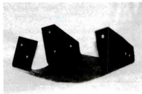
far into the radio chassis, and then de-burred with the Dremel grinding stone. I purchased four nylon spacers and cut them to size to center the rig into its new home. While doing a trial fitting, I mounted the microphone clip using one of the Yaesu mounting bolts, and marked where I would have to drill my final hole to finish the rack.
