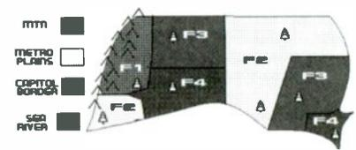
tem radio zones are established, there are still "dead areas" in various parts of a radio zone. These can be due to any one of a number of factors: The radio zone is still too big and parts of the radio zone are over the radio horizon, mountains are in the way, or big buildings in a city block the radio signals. Since subdividing radio zones and establishing new dispatch centers is not an economical or effective response, several different solutions are used.
