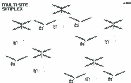
In this type of system every base and mobile shares the same radio frequency and every unit can hear every other unit and base station within range.
