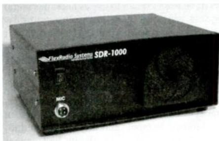
*The FlexRadio SDR-1000 is the first commercially available Amateur Band Software Defined Radio*
