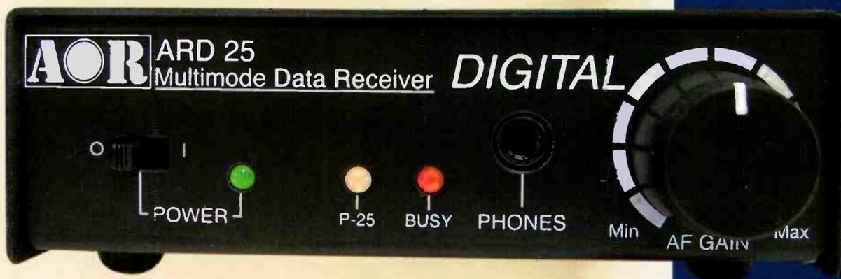
*Many high quality receivers were "left behind" when some public agencies began to use APCO Project 25 digital modulation. If your receiver has a 10.7 MHz output port, the ARD25 can translate those digital signals to intelligible audio. In addition, you can also channel your receiver's analog output through the ARD25. It will automatically recognize analog signals and pass them to the ARD25 internal speaker or to an external station speaker.*
