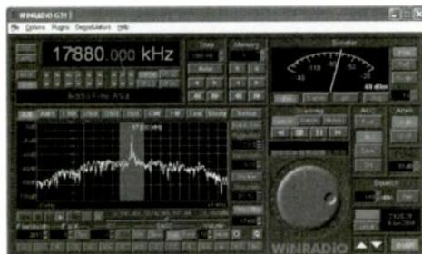
Now available in two models, the G313i (PCI card) and G313e (external USB module) offer continuous 9 kHz-30 MHz frequency coverage (optionally extendable to 180 MHz) with incredible signal-handling flexibility! Ideal for professional signal surveillance.
