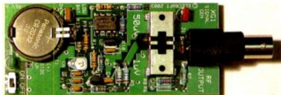
Figure 4 - Elecraft's XG-1 - The \$39(!) precision signal and level calibrator (after assembly)
