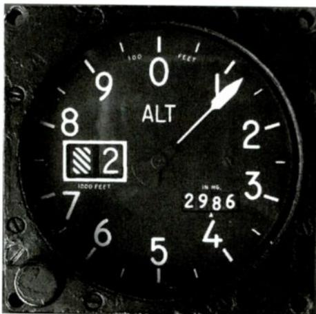
*This altimeter reads just short of 2,125 feet MSL. The altimeter setting / barometric pressure is set for 29.86. The adjustment knob is at the bottom left corner.*
