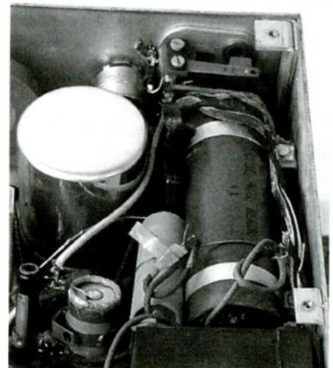
Cobbled-up replacement of multisection filter cap in original radio. Factory capacitor, abandoned in place, is large cylindrical unit at right.
