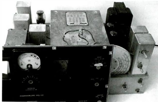
Original radio with cabinet and panel removed. Note warped section of bandspread dial (to right of panel top corner) and resistors wired into dial lamp circuit.
