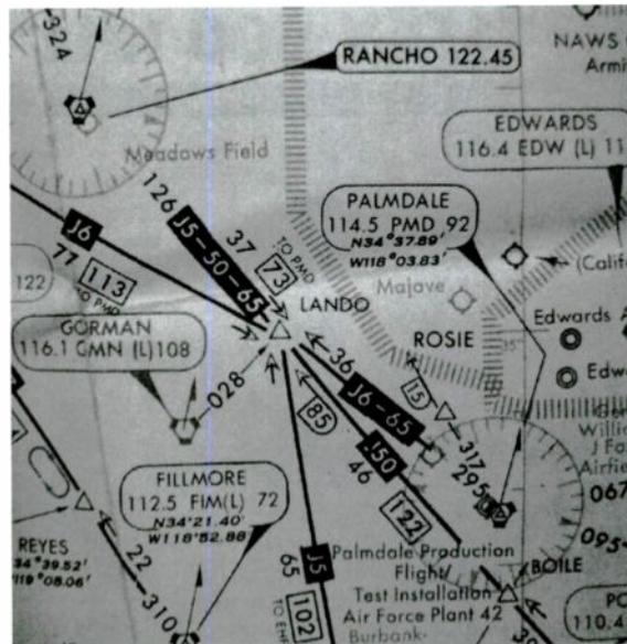
*This is the Lando intersection on the IFR ENROUTE HIGH ALTITUDE H-2 Chart. Note the Jet Routes J5, J6, J50, and J65 passing through this intersection.*
