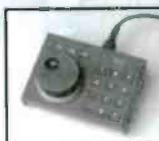
Allows armchair tuning of the RX-350D. Function buttons allow operation of various receiver controls. Direct frequency entry via keypad.
