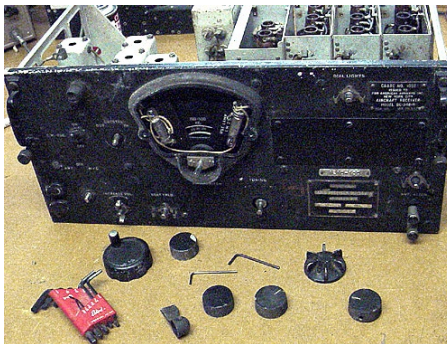
All knobs were taken off as first step in removing front panel.
