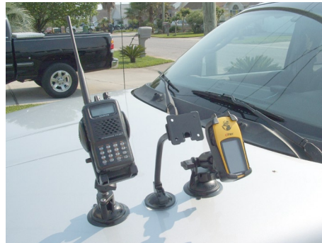
Three suction-cup mounts: Left to Right: RAM-Mount Universal Mount, Bracketron GNSM Flexible Mount, RAM-Mount for eTrex
