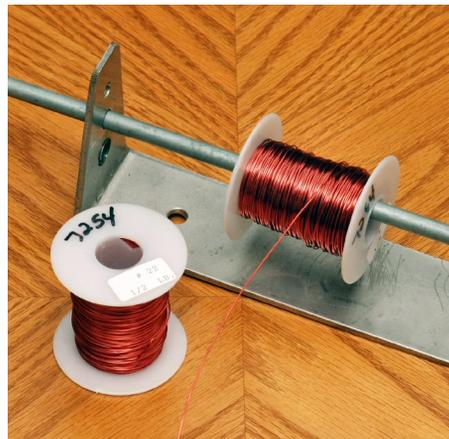
Figure 2. Spools of magnet wire and a simple but helpful holding device.
