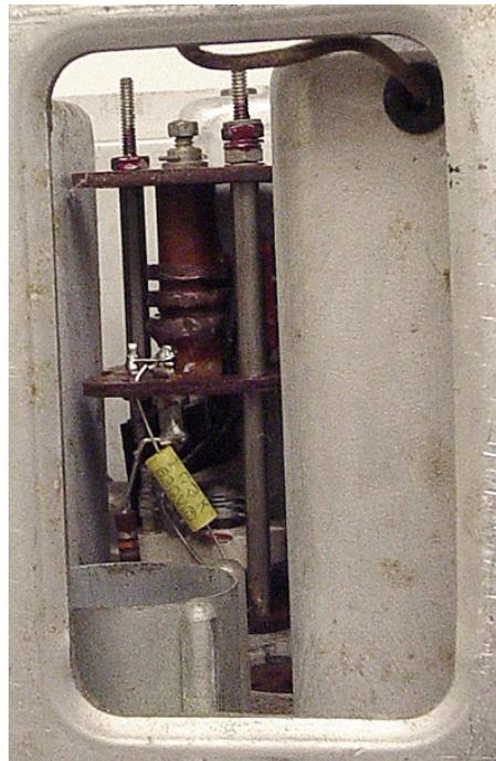
Peeking between a couple of shield cans at the opened c.w. oscillator gives us a view of the replaced paper capacitor.
