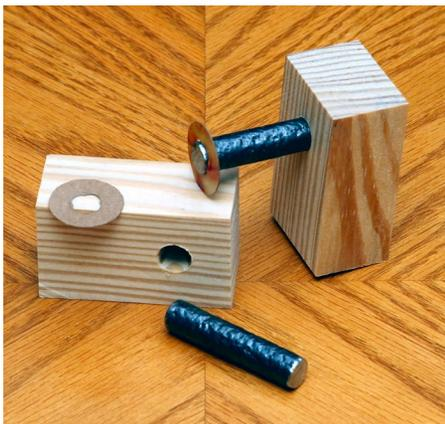
Figure 4. Field cores and wooden supports.
