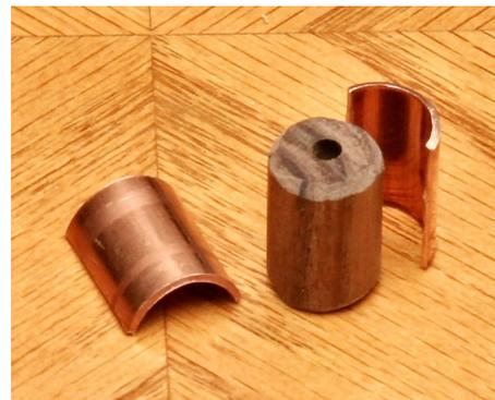
Figure 6. Commutator pieces before gluing.
