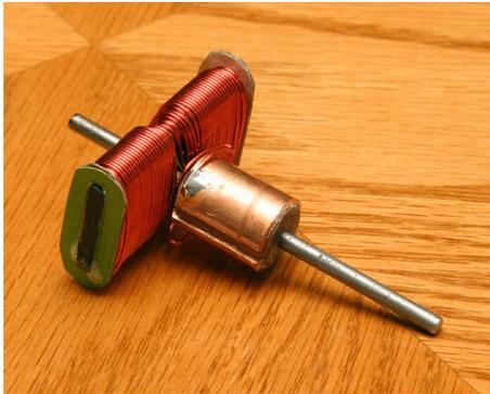
**Figure 7. Completed armature with commutator connected by soldering.**
