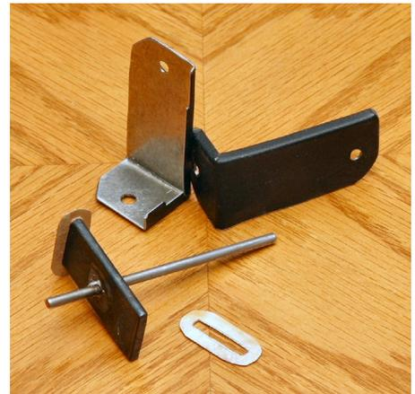
Figure 3. The soldered armature core and metal supports.
