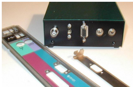
Photo A. CPU facing in color, stainless video card mount strip, and completed rear of project.
