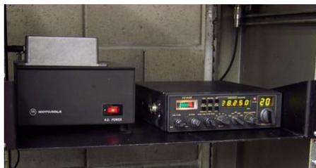
**K6FRC/B3 uses a VR-900 radio with a PicCon controller. (Courtesy: Paul Shinn K6FRC)**
