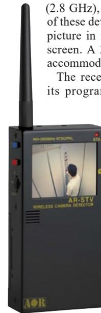
Detectable formats include NTSC, PAL, CCIR, EIA, and scrambled/reverse polarity video signals often encountered on 1.2 GHz L band and 2.4 GHz S band (WiFi). Typical sensitivity is -80 dBm @ 2.4 GHz.
