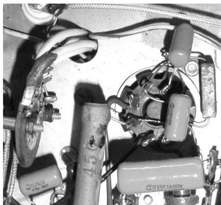
Under the 6146 tube socket, showing four of the replaced .005 uf capacitors. The larger one is a 1600-volt unit, replacing the original 1000-volt capacitor.
