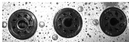
*After cleaning, the chassis proved to be covered with spots where the plating had been attacked. But at least there was no rust.*
