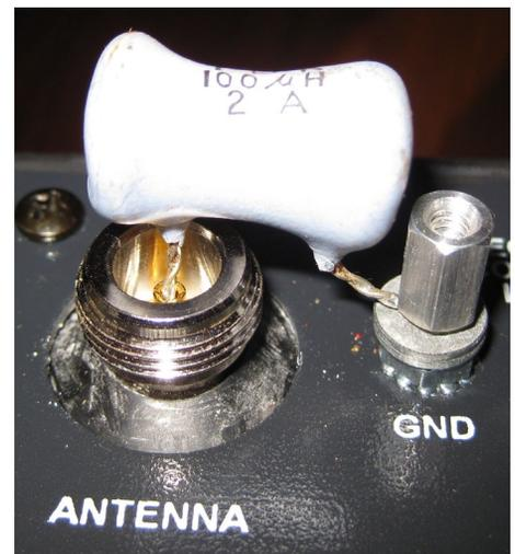
If you make the measurement at the end of a length of coax, you must subtract the coax distributed capacitance from the displayed value. The coax capacitance is revealed on the display before connecting the capacitor.
